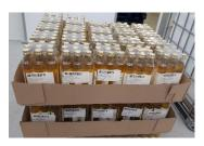
Consequently, pallet sizes have increased to 810 bottles, almost twice the quantity compared to the 480 bottles per pallet used by the manual system. However, the new automated system is unable to cope with the cardboard packaging, so a new packing system has been developed to cope with the larger pallet sizes. This involves shrink wrapping batches of 9 bottles together to protect them.
