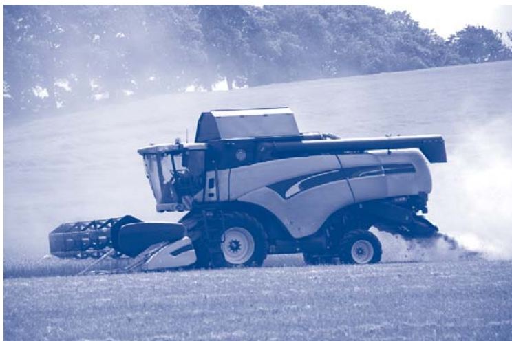
After winnowing inside the harvester, chaff is blown out.
